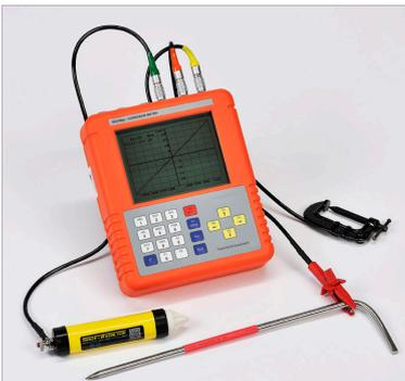
The test is carried out automatically by the BGCMAP, which applies a current and records the voltage. The GPS co-ordinates and the date and time of the test are also recorded. polarisation resistance (R<sub>p</sub>).
